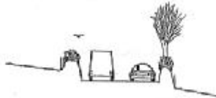
Figure 4.11 Typical cross-section of a Traditional A/B road. Typical width excluding verges = 6m. Total length = 1,521 km
